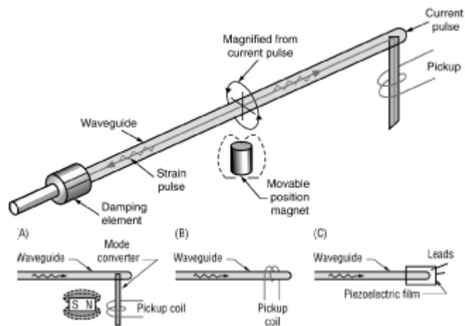
that is mounted within a protective housing made of a non-magnetic material. The waveguide is spring mounted on one end for damping. An external magnet moves along the exterior of the housing.
